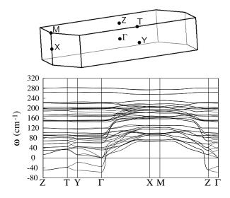
FIG. 2. (Top) The Brillouin zone of orthorhombic  $Ta_2NiSe_5$ . (Bottom) Calculated phonon dispersions of fully-relaxed orthorhombic  $Ta_2NiSe_5$  obtained using the optB88-vdW functional.
