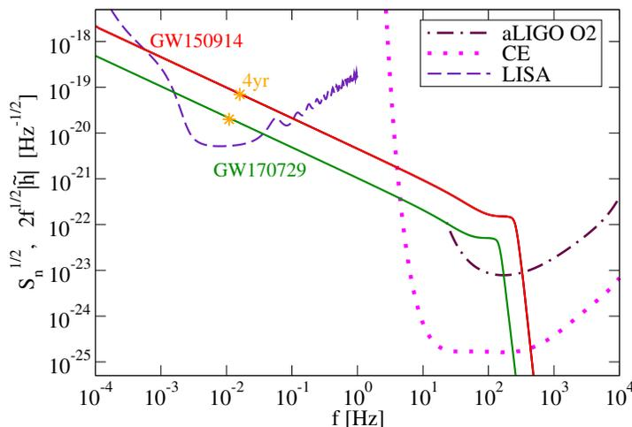
**Figure 1.** Sensitivities  $\sqrt{S_n(f)}$  of the gravitational-wave interferometers aLIGO O2, CE, and LISA considered in this analysis. We additionally display the characteristic amplitudes  $2\sqrt{f}|\tilde{h}(f)|$  for GW events GW150914, and GW170729 with 4 years prior to merger displayed as orange stars.
