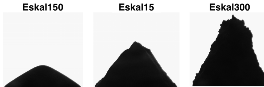
Figure 4: Typical heaps obtained with Eskal150, Eskal15 and Eskal300.
