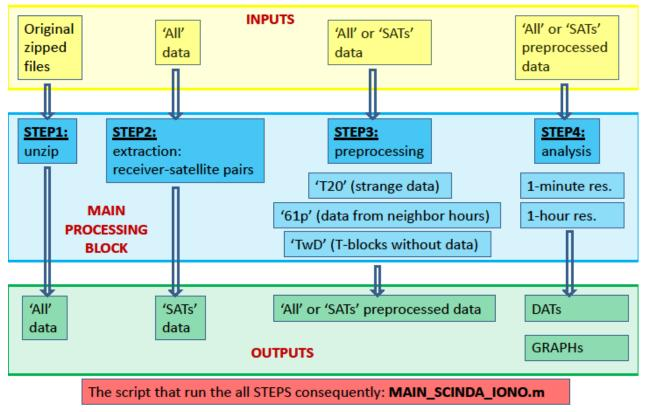
Figure 7: "SCINDA-Iono" toolbox architecture.
