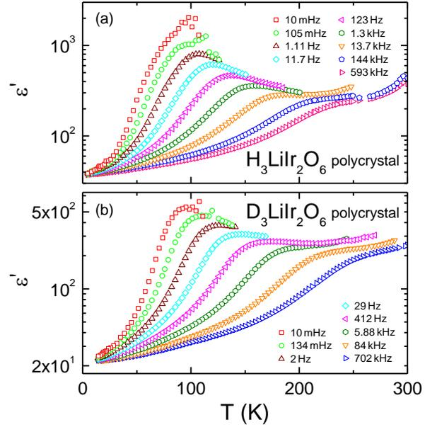
FIG. 3. Temperature dependence of the real part of the dielectric constant  $\epsilon'$  in (a) polycrystalline  $\text{H}_3\text{LiIr}_2\text{O}_6$  and (b) polycrystalline  $\text{D}_3\text{LiIr}_2\text{O}_6$  shown for a series of measuring frequencies.
