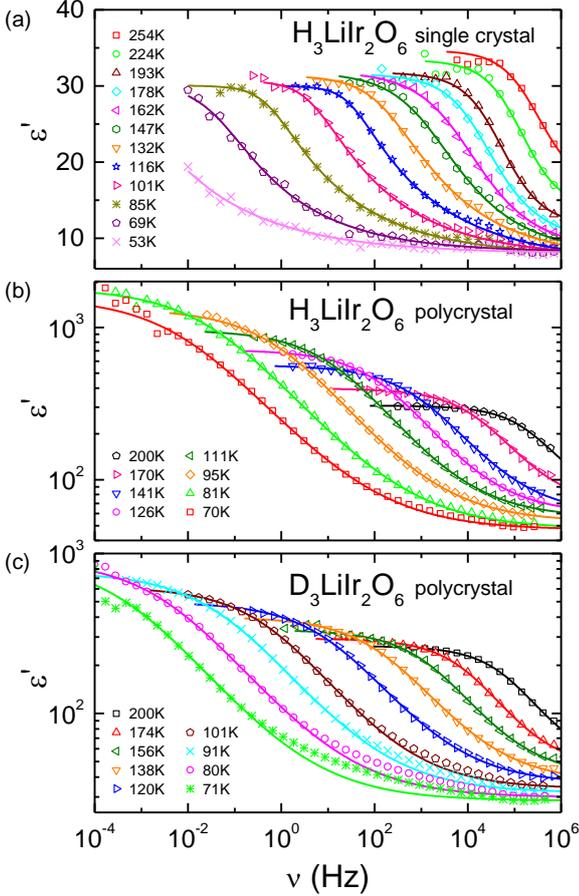
FIG. 4. Frequency dependence of the dielectric constant  $\epsilon'$  for (a) single crystalline and (b) polycrystalline  $\text{H}_3\text{LiIr}_2\text{O}_6$ , as well as for (c) deuterated polycrystalline  $\text{D}_3\text{LiIr}_2\text{O}_6$ . Data within the frequency region dominated by the observed relaxation processes are shown for selected temperatures as indicated in the frames. The lines represent fits using the Havriliak-Negami formula, Eq. (1), as described in the text.
