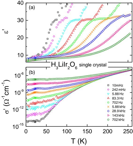
FIG. 2. Temperature dependence of (a) the real part of the dielectric constant  $\epsilon'$  and (b) the real part of the conductivity  $\sigma'$  as measured in single-crystalline  $\text{H}_3\text{LiIr}_2\text{O}_6$  shown for a series of frequencies.
