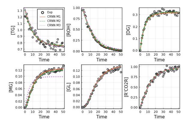
**Figure 9.** The noisy species concentration profiles and the predictions using the learned CRNN models. M1 corresponds to the CRNN learned from complete dataset, M2 corresponds to the CRNN learned from incomplete dataset with DG included in the CRNN inputs and outputs, and M3 corresponds to the CRNN learned from incomplete dataset but excluding DG from the CRNN inputs and outputs.
