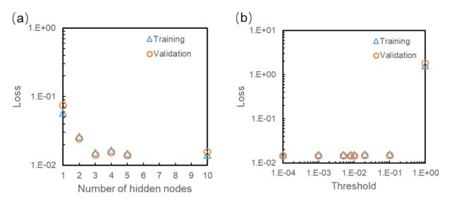
**Figure 7.** The dependence of minimum loss functions for the training and validation dataset with (a) the number of hidden nodes and (b) the pruning threshold.
