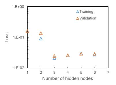
Figure. S2. The dependence of minimum loss functions for training and validation dataset with the number of hidden nodes.
