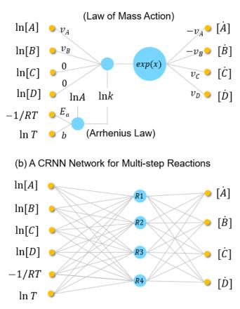
**Figure 1.** Schematic of the Chemical Reaction Neural Network illustrated for a reaction system with four species and four reaction steps. (a) First, a neuron is designed based on the Law of Mass Action and the Arrhenius Law, such that the learned neural network can be translated into interpretable reactions corresponding to the traditional chemical reaction network. (b) Then, the neurons are stacked into one hidden layer to formulate a CRNN for multi-step reactions.
