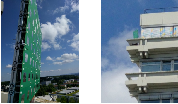
Fig. 6: Photos of basestation receiver antenna with 64 antenna elements
