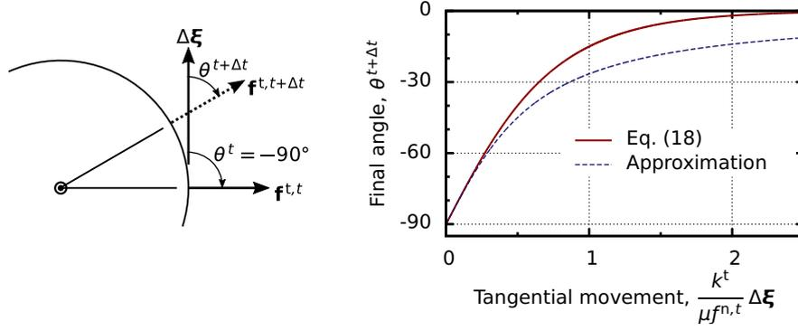
**FIGURE 4** Example showing the effect of the magnitude of the tangential movement  $\Delta\xi$  on the final direction of the tangential force. The movement  $\Delta\xi$  is applied orthogonal to the initial force  $\mathbf{f}^{t,t}$ .
