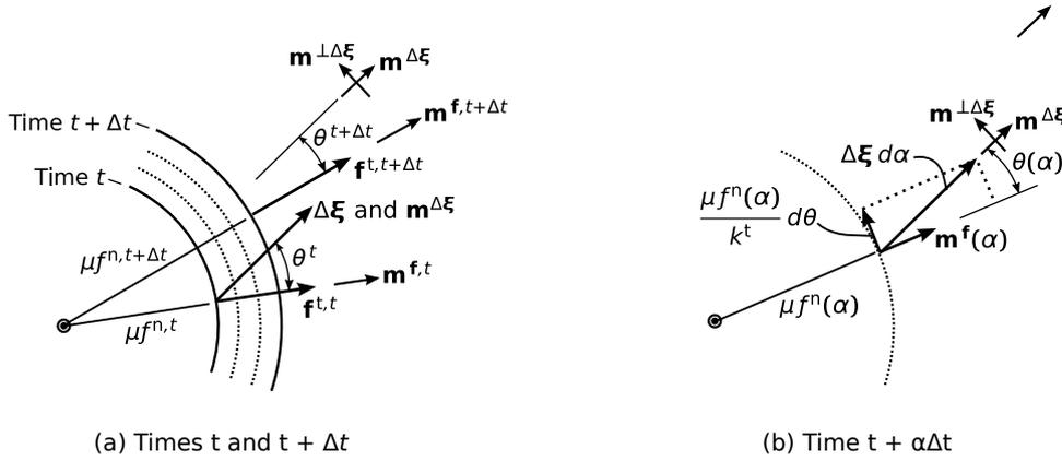
**FIGURE 3** Evolution of the tangential force and sliding direction: (a) yield surfaces and the initial and final directions of the tangential force, and (b) increment in movement tangent to the yield surface. Note that the  $\theta$  angles are negative in the directions of this figure.
