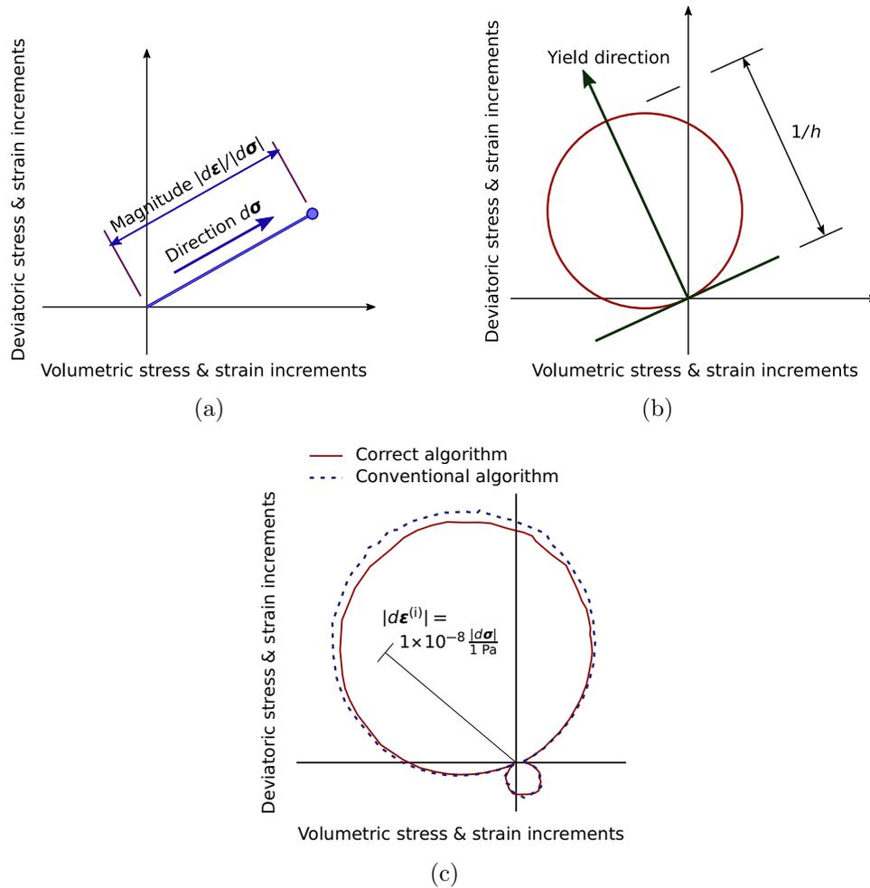
**FIGURE 5** Plots of incremental plastic strains from stress-probes in the Rendulic plane of volumetric and deviatoric stress and strain: (a) technique for plotting the plastic increment of a single probe; (b) locus of probe points, as predicted by elasto-plastic theory; and (c) locus of probe points for two the linear-frictional algorithms.
