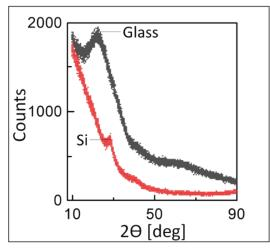
Figure S1| X-ray diffraction of amorphous molybdenum silicide. XRD profile of a 15-nm thick  $\alpha$ Mo<sub>81</sub>Si<sub>19</sub> film on glass (black) and silicon (red) substrates. Peak of the silicon substrate and low-angle broadening due to the glass substrates are highlighted. The absence of any other significant peaks indicates on the amorphous nature of the films.
