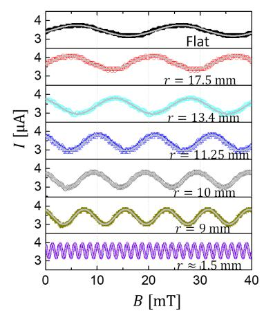
**Figure S3** Effects of bending on interference periodicity in flexible SQUIDs for a large set of curvatures. Interference pattern of SQUIDs with varying radii of curvature (marked in the figure). Gray lines are the best fits for a sine function. The fitting parameters are given in Table S1.
