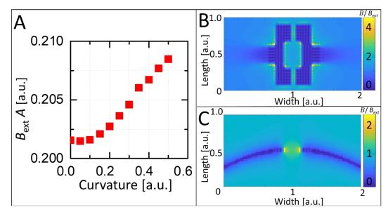
**Figure S7 Contribution of lensing effects on magnetic-field enhancement.** (**A**) Calculated maximal magnetic-field augmentation due to lensing for various curvatures. (**B**) top and (**C**) side view of the simulated magnetic-field enhancement in a device with a substantial curvature (orders of magnitude larger curvature than in our experiments), showing enhancement that is much lower than the observations. Simulations follow Reference (*31*).
