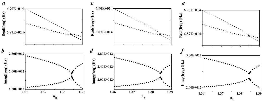
Figure S2. The real and imaginary parts of eigenvalues for the system with intrinsic losses. The refractive index of  $\text{Si}_3\text{N}_4$  is chosen as  $n=2.02+0.003i$  for (a) and (b),  $n=2.02+0.004i$  for (c) and (d) and  $n=2.02+0.005i$  for (e) and (f).
