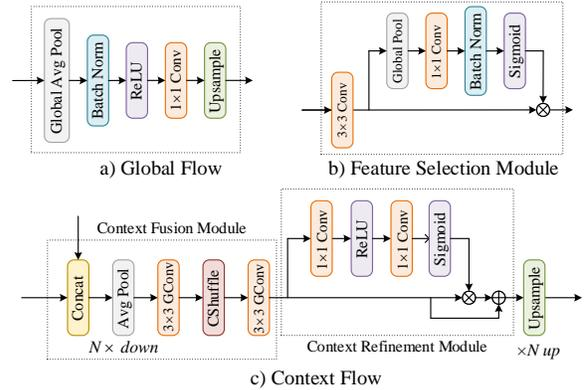
Figure 3. Detailed components of CAM. “ $N \times$  down” means  $N$ -time downsampling of the inputs by average pooling layer, while “ $\times N$  up” means  $N$ -time upsampling operation. GConv and CShuffle are shorthand for Group Convolutions and Channel Shuffle respectively.  $\oplus$  and  $\otimes$  represents element-wise summation and element-wise product, respectively.
