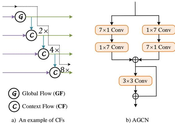
Figure 4. a) One possible combination of GF and CFs. “ $N \times$ ” indicates the down-sampling rate of the pooling layer in CFs. b) Skip connection in decoder that employs large-kernel convolutions adapted from Global Convolutional Network, which we referred to as AGCN.  $\oplus$  is element-wise summation.
