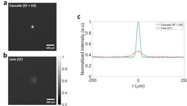
**FIG. 5** a) The confined beam profile of light at the optical depth of 4.38 TMFP into the scattering medium using a cascade system of an aspheric lens with a short focal distance (SF)  $f = 25$  mm (measured in air) and the virtual GRIN waveguide formed at  $d_o = 13.47$  mm. b) The confined beam of light using a single aspheric lens with a longer focal distance (LF)  $f = 50$  mm (measured in air). c) Radial cross-sections of the beams for the single external lens and the cascade system.
