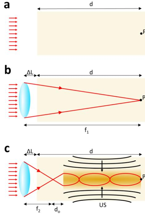
**FIG. 1** a) Schematic illustration of a collimated beam of light from an external source and the target point  $P$  inside the medium. b) An external lens with a long focal distance ( $f_1$ ) is used to focus light to the target location  $P$  at a depth  $d$  inside the medium. c) A cascade optical system of an external lens with a short focal distance ( $f_2$ ) and an ultrasonically defined virtual GRIN waveguide is used to relay the focused spot through the medium to the same point  $P$ .
