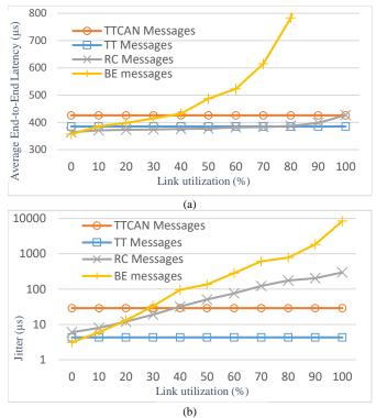
Fig. 6. The influence of link utilization on (a): average end-to-end latency performance and (b): the jitter performance of all traffic.
