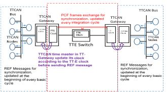
Fig. 5. An example of interworking between TT-E and TT-CAN protocols via a TT-Gateway.
