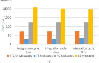
Fig. 7. The impact of the integration cycle on (a): throughput performance and (b): jitter performance.
