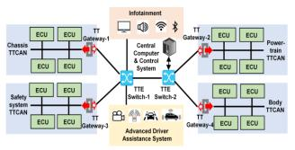
Fig. 1. A simplified in-vehicle time triggered communication system.
