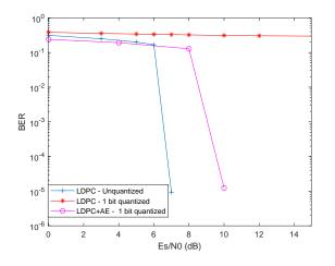
Fig. 3. The error rate for the code rate  $\frac{1}{2}$  LDPC code with a codeword length of 64800 bits for 16-QAM
