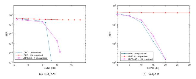
Fig. 2. The error rate for the code rate  $\frac{1}{2}$  LDPC code with a codeword length of 648 bits
