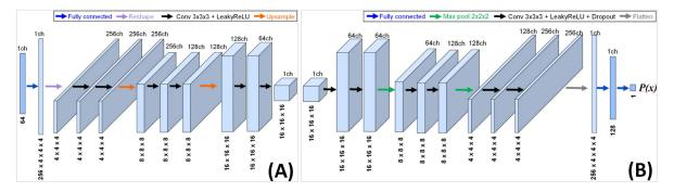
Fig. 2 The generator (A) and discriminator (B) networks of the used 3D DCGAN.
