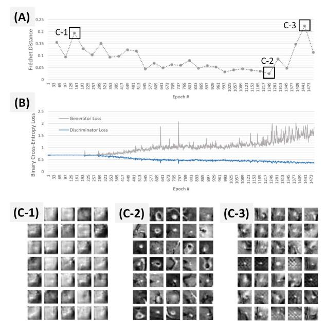
Fig. 4 Fréchet Distance (FD) for the GAN validation.
