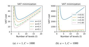
Figure 2: (a) VAT cost ratio  $(T/T_{opt})$  for optimal throughput (r = 1) and different values of merge amplification *a*. (b) VAT cost ratio at maximum merge amplification (a = 1) and different values of achieved device throughput *r*.
