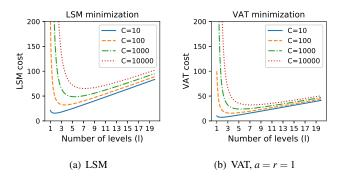
Figure 6: (a) Amplification vs. number of levels as a result of minimizing the LSM cost for various  $C = \frac{Workload \ size=S_I}{DRAM \ size=S_0}$  ratios. (b) Amplification vs. number of levels as a result of minimizing VAT cost for various *C* ratios.
