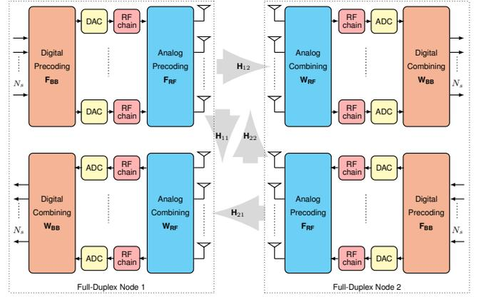
Fig. 1. Architecture of a hybrid two-node FD network.
