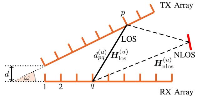
Fig. 2. Relative position of TX and RX arrays at FD node  $u$ . Given that the TX and RX arrays are collocated, the far-field assumption that the signal impinges on the antenna array as a planar wave does not hold. Instead, for FD transceivers, it is more suitable to assume that the signal impinges on the array as a spherical wave for the near-field LOS channel.
