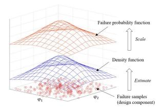
Figure 1: Estimated density function and the corresponding failure probability function
