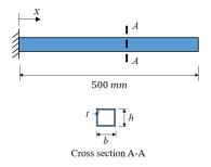
Figure 5: Diagram of the studied cantilever box beam
