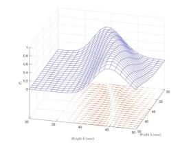
Figure 8: Approximated failure probability funciton and the vector field of its gradient
