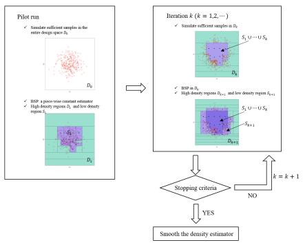
Figure 2: An iterative scheme for density estimation
