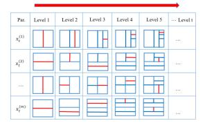
Figure 3: Sequential partitioning process of BSP (in each level, a total number of m partitions are simulated)
