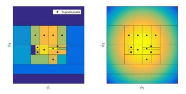
*Figure 4: Smoothing of a piece-wise constant estimator (left panel: piece-wise constant estimator; right panel: smoothed estimator)*
