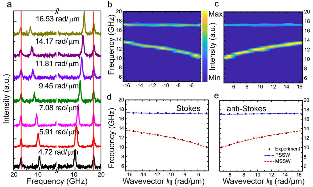
**Figure 2 .** a) BLS intensities spectra of Ni<sub>79</sub>Fe<sub>21</sub> (34 nm) film for different wavevectors  $k_{||}$  with  $\mathbf{H} = 500$  Oe. Red vertical lines corresponding to 1st PSSWs. Density plot of BLS intensity in  $\omega$ - $k$  plane: b) Stokes and c) anti-Stokes. Dependence of the spin waves frequency on the transferred wave vector  $k_{||}$ : d) Stokes and e) anti-Stokes. The dashed red line is the MSSW band  $f_M$ . The dash-dotted blue line is the 1st PSSW  $f_P^1$ .
