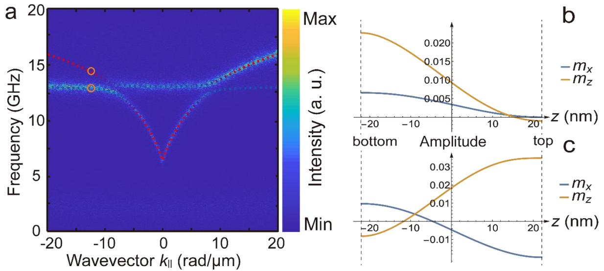
**Figure 4.** a) The simulation results of Ni<sub>79</sub>Fe<sub>21</sub> (44 nm) film. The gradient blue and red lines are the theoretically derived dipole-exchange bands. The density plot is the micromagnetic simulation result. b) and c) The wavefunction amplitudes of  $k_{||} = -12 \text{ rad}/\mu\text{m}$  of (b) the higher-frequency band (MSSW branch) and (c) the lower-frequency band (PSSW branch).
