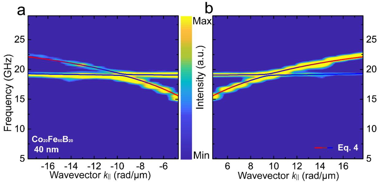
**Figure 5 .** a) and b) Density plot of BLS intensities spectra of  $\text{Co}_{20}\text{Fe}_{60}\text{B}_{20}$  (40 nm) film in  $\omega$ - $k$  plane with  $\mathbf{H} = 500$  Oe: a) Stokes and b) anti-Stokes. The gradient solid lines are given based on the two-band model (Equation 4).
