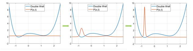
Fig. 3. Time evolution of Quantum Annealing process for optimization of a function having both local and global optimum
