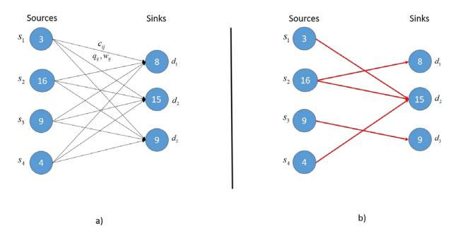
*Fig. 10. a) Minimum number of matches problem and b) Obtained optimal solution for the problem instance*
