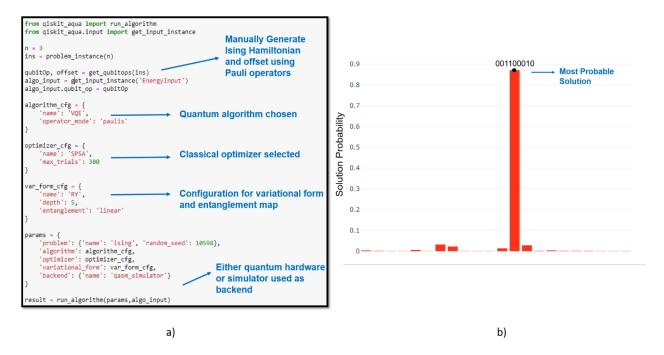
*Fig. 5. a)* Python code sample showing the use of Qiskit to solve a problem instance, and b) Histogram representing likelihood of possible solutions
