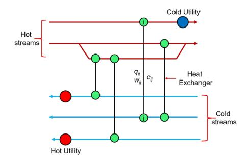
Fig. 9. Heat exchanger network containing 2 hot streams and 3 cold streams
