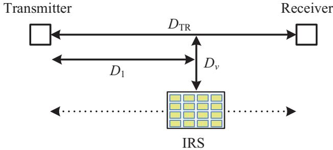
Fig. 3: Simulation setup.
