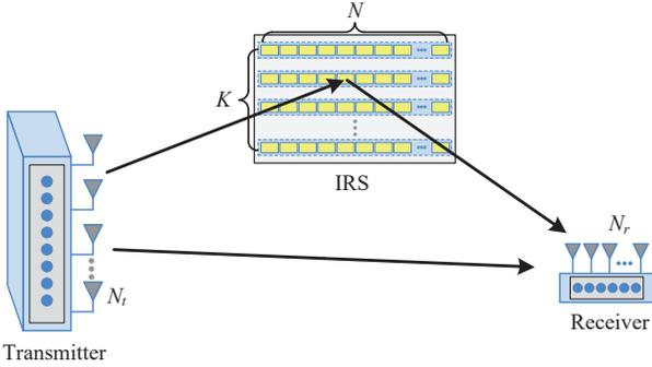
Fig. 1: IRS-assisted mmWave massive MIMO single-user system
