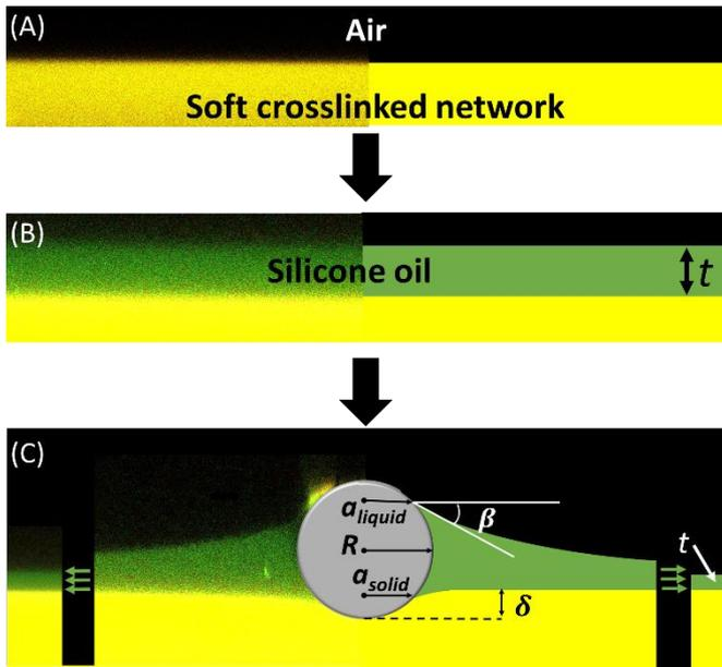
Figure 1. Confocal images (left) are shown alongside schematics (right) of (A) a cured 60 to 1 Sylgard 184 substrate shown in yellow, (B) the substrate with an oil layer shown in green, and (C) the oil-coated soft substrate with a microsphere placed on the surface. In (C), the green arrows denote a distance far from the particle. The schematics provide descriptions of the variables measured from the images.
