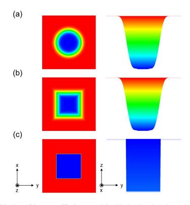
**Figure 3.** Top-view and Side-view of the EMA effective potentials with the shape based on (a,b) DFT KS potential and (c) abrupt step-potential. Radial smoothened DFT KS potentials shown in figure 2(c) were directly converted into (a) cylindrical and (b) rectangular potential shape.
