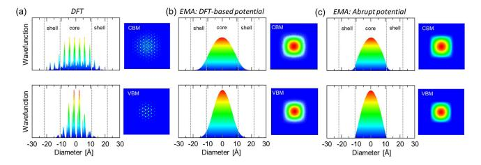
**Figure 4.** The radial cross-sectional view of the electron (top) and hole (bottom) wavefunctions of CdS/ZnS core/shell nanostructures generated within (a) DFT, (b) DFT-KS potential based EMA and (c) abrupt potential based EMA.
