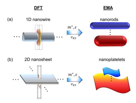
Figure 1. Schematics of the proposed DFT-based EMA calculation strategy. For the (a) nanorod and (b) nanoplatelet cases, e.g., we perform DFT calculations for the corresponding ideal 1D nanowire and 2D nanosheet or slab, respectively, and extract the nanoscopic electron/hole mass  $m_{e/h}^*$ , dielectric constant  $\epsilon$ , and the confinement potential profile  $v^{KS}$  for EMA calculations.
