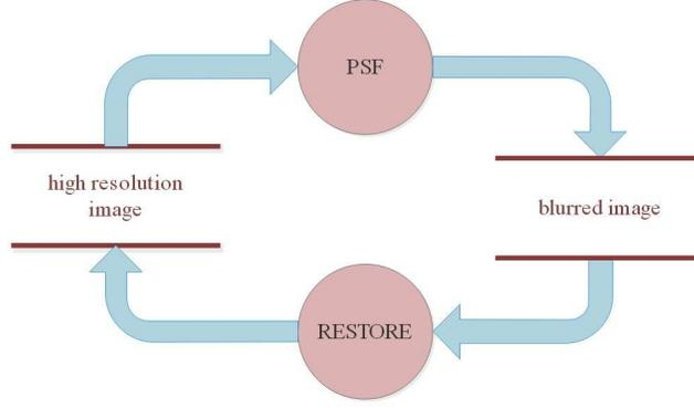
**Figure 2.** The overall structure of PSF-NET. The PSF network is used to model the PSF, which transforms high resolution images into blurred images. The RESTORE network is used to model deconvolution kernel, which transforms blurred images into high resolution images.
