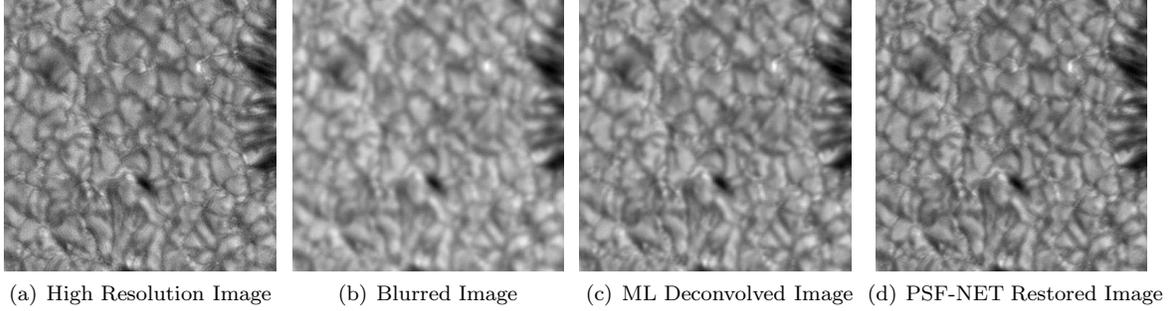
**Figure 6.** (a) is the original high resolution H-alpha wavelength image, (b) is the simulated blurred image, (c) is the image restored by the maximum likelihood (ML) blind deconvolution algorithm in the MATLAB and (d) is the image restored by the RESTORE in a trained PSF-NET.
