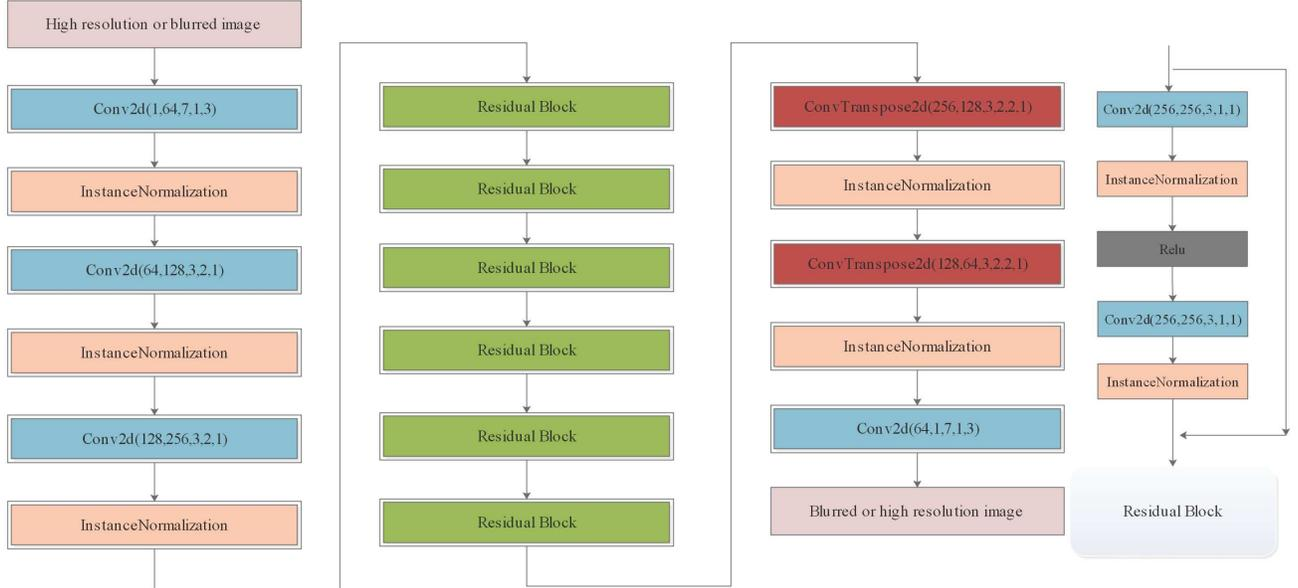
**Figure 3.** A structure diagram of a CNN, which could either be the PSF or the RESTORE. This CNN consists of convolutional layers (Conv2d in blue), instance normalization layers (IN in pink), Conv-transpose layers (ConvTranspose2d in red) and Residual blocks (Residual block in green). The structure of residual block is shown on the right. The Relu layer in gray color is used in the residual block as activation function.
