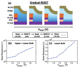
**Figure 10**. (a) The schematic showing gradual filling of the oxygen vacancies (shaded region) due to gradual RESET (by  $V_{RESET}$ , (b) gradual resistance increase in the upper + lower bulk region of the device with  $V_{RESET}$  (c) gradual resistance change in the lower bulk region of the device  $V_{RESET}$ . A large change in the upper bulk region is observed owing to the higher trap density in the upper bulk region.
