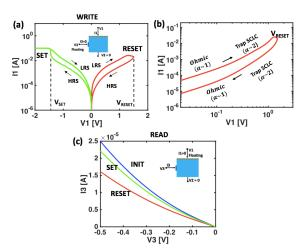
**Figure 7**. (a) WRITE: Typical dciv of the PCMO RRAM showing the SET and RESET on opposite polarities. The inset shows that the bias is applied between T1 and T2, (b)log-log dciv on the positive polarity showing the SCLC mechanism, (c) READ: V3 vs. I3 showing the change in the current which indicates the resistance change in the lower bulk region of the device.
