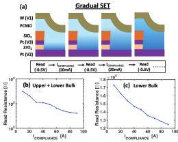
**Figure 11**. (a) The schematic showing gradual filling of the oxygen vacancies (shaded region) due to gradual SET (by current compliance), (b) gradual resistance decrease in the upper + lower bulk region of the device, (c) gradual resistance change of the lower bulk region of the device. A large change near the upper bulk region is observed owing to the higher trap density in the upper bulk region.
