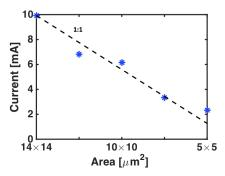
Figure 6. Current (Between T1 and T2) vs. Area of the PCMO devices showing the  $\sim 1:1$  relation to the current and area indicating the current scaling with the area, a signature of the non-filamentary nature of the device.
