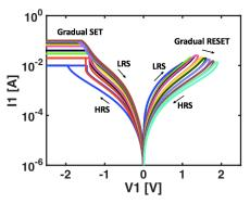
**Figure 9**. A Gradual change in resistance from LRS to HRS (by  $V_{RESET}$ ) and from HRS to LRS (by current compliance).
