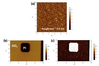
**Figure 4**. (a) AFM showing PCMO film roughness ~0.9nm, (b) AFM and (c) its phase image of OMO layer after step 2 (Figure 2) indicates two different surfaces (Pt and SiO<sub>2</sub>).
