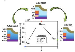
**Figure 8**. Read resistance of the PCMO device with a schematic showing the oxygen-rich or poor regions in the PCMO film after the application of SET and RESET bias.
