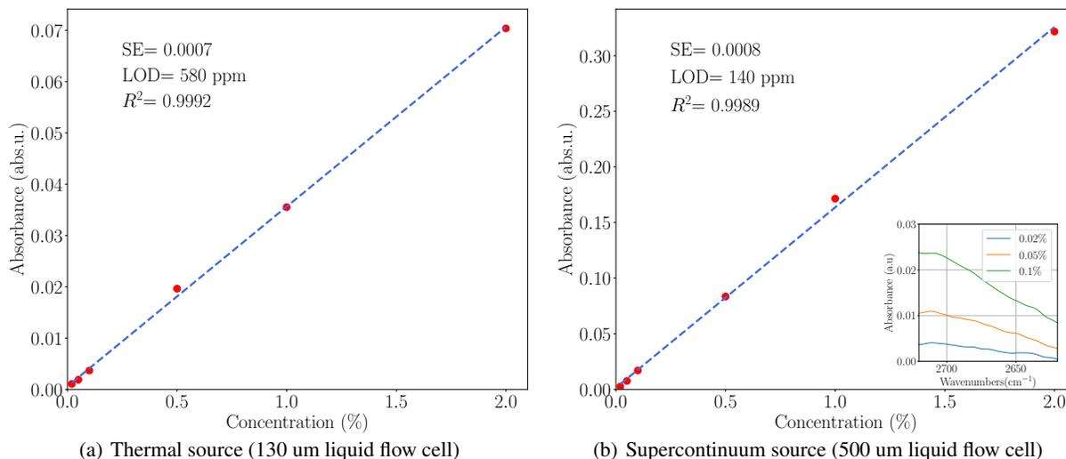
Figure 7: Calibration curves of a formaldehyde (methanediol) dilution series obtained by integrating the absorbance within the spectral range of  $2720\text{ cm}^{-1}$  -  $2620\text{ cm}^{-1}$ , covering parts of the C-H stretching band (a) standard FTIR instrument with CW thermal emitter and  $130\text{ }\mu\text{m}$  optical path length flow cell; (b) supercontinuum-based FTIR and  $500\text{ }\mu\text{m}$  flow cell.
