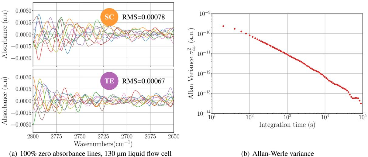
Figure 5: (a) Noise performance of the experimental setup using a 130  $\mu\text{m}$  liquid flow cell filled with blank water: the supercontinuum source (marked as SC) in comparison to the thermal emitter (TE) expressed in the form of 100% (zero absorbance) lines and (b) long-term stability of the LIA based setup illustrated by the Allan Werle variance.
