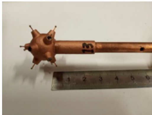
Figure 2. ACHINOS using an Araldite-copper layer on the 3-D-printed structure to form the central electrode.
