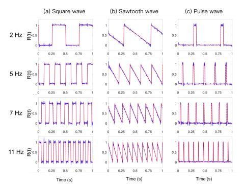
Fig. 3. Reconstructed ghost images of basic function waveforms. (a) Square wave. (b) Sawtooth wave. (c) Pulse wave. The frequencies of the signals are 2, 5, 7, 11 Hz from top to bottom, respectively. Blue solid lines: reconstructed ghost images. Red dash lines: ground truth references.
