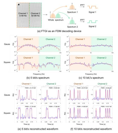
Fig. 8. Demonstration of FDM decoding. (a) Illustration of FDM decoding. (b) Spectrums of 5 bit/s gauss and square RZ signals. (c) Spectrums of 10 bit/s gauss and square RZ signals. (d) Reconstructed waveforms of 5 bit/s gauss and square RZ signals. (f) Reconstructed waveforms of 10 bit/s gauss and square RZ signals. Blue solid lines: reconstructed ghost images. Red dash line: ground truth references.
