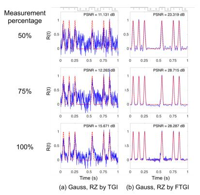
Fig. 7. Comparison between TGI and FTGI results. Blue solid lines: reconstructed ghost images. Red dash line: ground truth references. (a) RZ Gauss code ghost image by TGI. (b) RZ Gauss code ghost image by FTGI.
