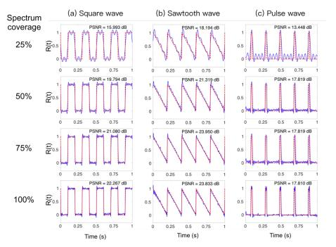
Fig. 4. Reconstructed ghost images with different spectrum coverage. The frequency of time objects is 5 Hz and the spectrum coverages are from 25% to 100% (top to bottom in the figure). Blue solid lines: reconstructed ghost images. Red dash line: ground truth references. (a) Square wave. (b) Sawtooth wave. (c) Pulse wave.
