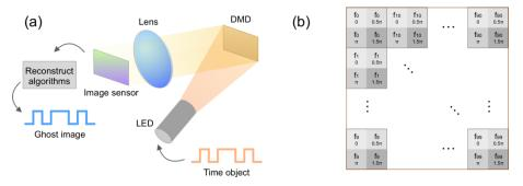
Fig. 1. Overview of FTGI. (a) Experimental setup. DMD: digital micro mirror device. LED: light-emitting diode. (b) An illustration of DMD encoding pattern with the corresponding frequencies and phases marked in each patch.
