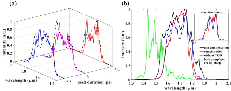
Fig. 4. (a) The output spectrum evolution with a seed pulse duration of 2.7 ps (blue solid line), 3.0 ps (pink solid line), and 3.4 ps (red solid line). Black dashed lines, simulation results. (b) The output spectrum with the influence of TOD and saturation effect in the OPA process. Black solid line, without TOD influence; blue solid line, with the TOD caused by the prism pair
