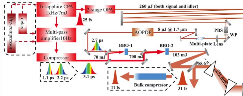
Fig. 1. Multi-TW few-cycle IR source based on DC-OPA; AOPDF, acousto-optic programmable dispersive filter, PBS, polarizing beam-splitter, WP, wave plate.
