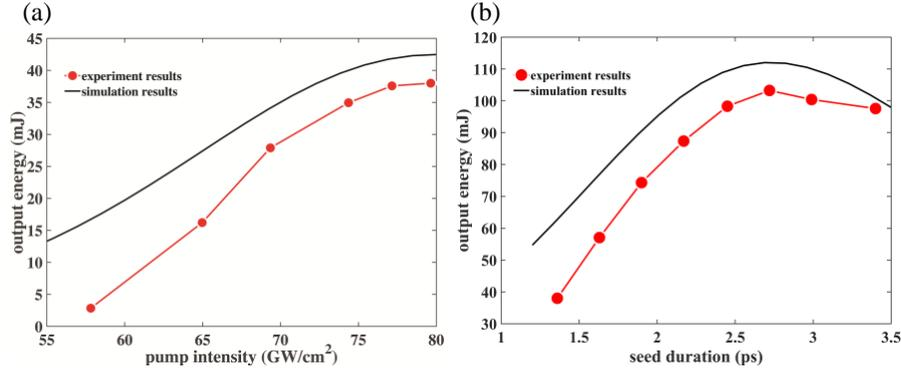
Fig. 3. The output energy after two stages of DC-OPA. (a) Energy scaling as a function of pump intensity. (b) Energy evolution as a function of seed pulse duration. Both in (a) and (b), the black solid line and red solid circles are simulation results and experiment results, respectively.
