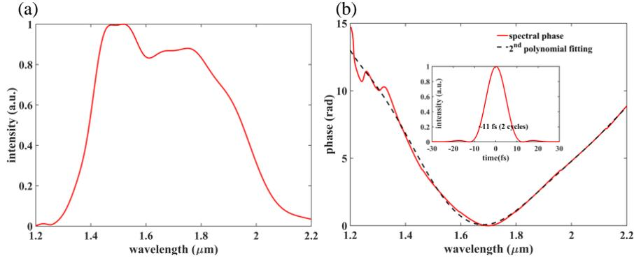
Fig. 7. (a) Simulation results of output spectrum after DC-OPA based on a dual pump DC-OPA scheme. (b) Simulation results of output spectral phase corresponding to the spectrum in Fig. 7(a) and compressed pulse duration with dispersion compensated.
