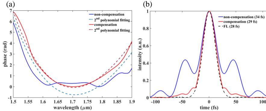
Fig. 5. (a) The simulation results of the output spectral phase caused by the DC-OPA process. Blue solid line, spectral phase corresponding to the simulated spectrum (blue solid line in the
