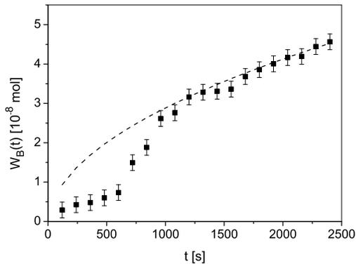
FIG. 3: Experimental results (squares) and theoretical function  $W_{B0}$  Eq. (25) (dashed line) for diffusion of ciprofloxacin through *P. mirabilis* O18 biofilm, fitting parameters are  $a_0 = 0.90 \times 10^{-5} \text{ m}/\sqrt{\text{s}}$  and  $b_0 = 0.95 \times 10^{-6} \text{ m/s}^{0.05}$ , and  $\alpha = 0.95$ ; here  $C_0 = 1.5 \text{ mol/m}^3$  and  $\Pi = 7.0 \times 10^{-5} \text{ m}^2$ .
