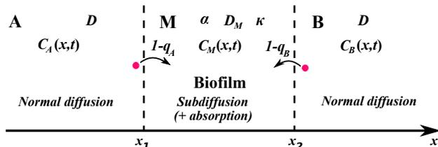
FIG. 1: Schematic of the system. The biofilm separates two regions in which normal diffusion occurs,  $D$  is the normal diffusion coefficients in regions  $A$  and  $B$ ,  $D_M$  is the subdiffusion coefficient,  $\alpha$  is the subdiffusion parameter and  $\kappa$  is the absorption coefficient in the biofilm,  $q_A$  and  $q_B$  are probabilities of stopping a diffusing particle by the biofilm boundaries.
