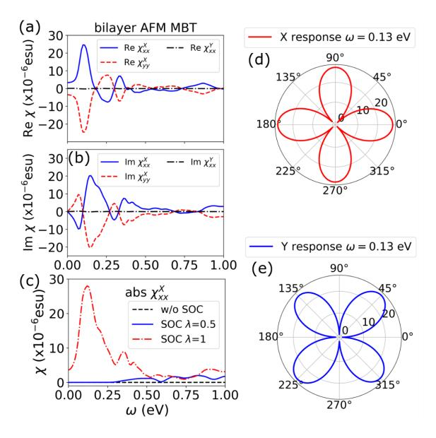
**Figure 4** (a) and (b) The real and imaginary parts of the SHG susceptibility tensor, respectively. (c) The absolute SHG susceptibility tensor  $\chi^{X}_{xx}$  for different SOC strength  $\lambda$ .  $\lambda = 1$  indicates the realistic case. (d) and (e) The *x*-direction and *y*-direction polarization component of the outgoing SHG response for different polarized incident photons at  $\omega = 0.13$  eV.
