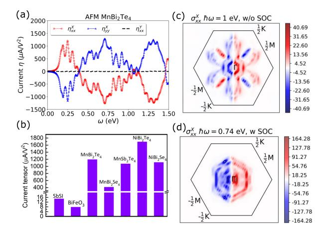
**Figure 3** (a) The linearly-polarized injection-current matrix element spectrum for bilayer MBT. (b) The maximal photocurrent response under linearly-polarized light for different MBT materials, bulk SbSI, [58] and BiFeO3 [55–57]. (c) and (d) The contour plots of first-principles calculated photoconductivity  $\eta_{xx}^{X}$  in the receiprical space without and with SOC, respectively.
