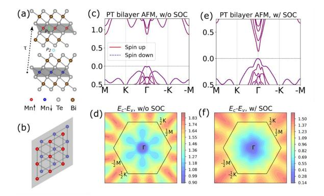
**Figure 1** (a) and (b) Side and top views of the atomic structure of AFM MBT crystal.  $\tau$  is the half translation,  $P_1$  is the inversion center of odd-number-layer AFM MBT, and  $P_2$  is the inversion center for even-number-layer MBT. (c) and (d) The band structure without and with SOC, respectively. (d) and (e) The energy difference between the LCB and HVB without and with SOC, respectively.
