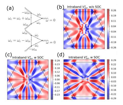
Figure 2 (a) The Feynman diagram for injection current. (b) and (c) The first-principles calculated intraband x-direction velocity matrix element without and with SOC, respectively. (d) That along the y direction with SOC.
