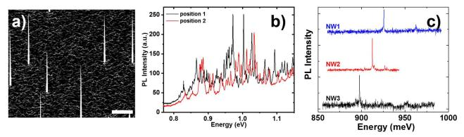
Figure 7. a) Typical tilted (45°) SEM image of low-density-needlelike-tapered InAs/InP QD-NWs with  $D_{NW} = 360$  nm at the bottom part of the NW and  $L_{NW} = 14$  µm. Scale bar is 5 µm. b) Low temperature (12 K) PL showing the emission lines from several InAs QDs at two different positions on the sample. c) Low temperature (12 K) micro-PL showing single emission lines from a single InAs/InP QD-NW.
