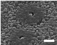
**Figure 5.** Tilted (45°) SEM image after 2 min growth of InP on a surface with droplets formed using the In/Au BEP ratio = 58, showing the formation of 3D islands of InP with the Au-In droplets having a diameter in the 400-500 nm range. Scale bar is 1  $\mu$ m.
