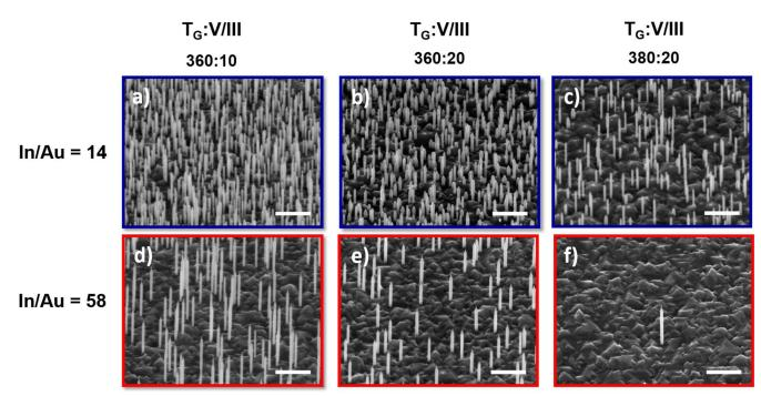
Figure 6. Tilted (45°) SEM images of the InP NWs grown at different growth temperature and P<sub>2</sub> BEP (or V/III BEP ratio), with In/Au BEP ratio = 14 (a to c) and In/Au BEP ratio = 58 (d to f). Scale bars are 1 μm.
