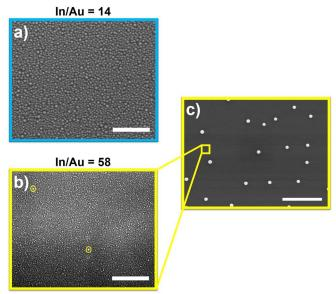
**Figure 3.** Top view SEM images of the Au-In droplets deposited at  $500^{\circ}$ C with an In/Au BEP ratio equal to: a) 14, b) 58 with the droplets in the yellow circles in the 20-40 nm diameter range. c) Low magnification image of the sample in (b) showing the droplet formation with diameter in the 400-500 nm range. Scale bars in (a), (b) 500 nm and (c) 5  $\mu$ m.
