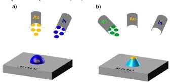
**Figure 1.** Schematic representation of : a) an Au-In core-shell droplet deposited at  $500^{\circ}$ C on Si(111) and b) an InP pedestal with an Au droplet on top after opening the  $P_2$  valve during 10 sec (from ref [18]).
