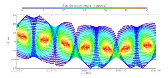
Figure 17. Coverage of the brightest limb tangent point in the atmosphere as seen by TGO. Latitudinal variation over time for 2020, with a sampling of 10 minutes. Coloured by solar elevation angle. (black is the minimum, limited to 10 degrees to avoid terminator; red is the maximum, 90 degrees at the sub-solar point)
