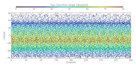
Figure 16. Coverage of the brightest limb tangent point in the atmosphere as seen by TGO. Latitude and longitude spatial coverage for the whole 2020, with a sampling of 10 minutes. Coloured by solar elevation angle. (black is the minimum, limited to 10 degrees to avoid terminator; red is the maximum, 90 degrees at the sub-solar point)
