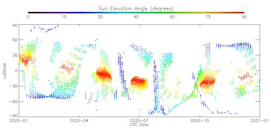
Figure 19. Latitude coverage over time of the simultaneous limb opportunities by MEX and TGO for 2019. Coloured by solar elevation angle. (black is the minimum, limited to 10 degrees to avoid terminator; red is the maximum, 90 degrees at the sub-solar point)
