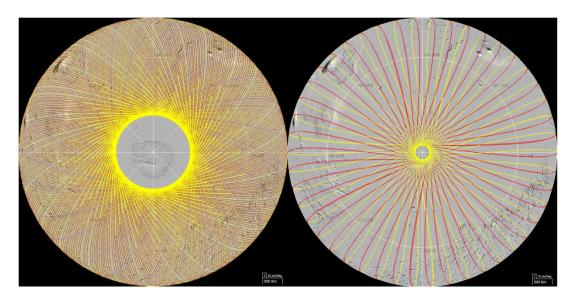
Figure 10. Four-week (one Medium Term Planning cycle) nadir ground-tracks of TGO (left) and MEX (right) in the northern hemisphere, as seen from the North pole. Dayside tracks are shown in yellow, nightside in red. MEX has a longer orbital period, therefore the surface coverage sampling is lower than TGO's.
