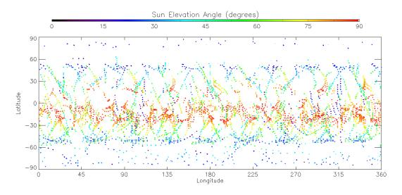
Figure 18. Spatial coverage (latitude vs longitude) of the simultaneous limb opportunities by MEX and TGO for 2019. Coloured by solar elevation angle. (black is the minimum, limited to 10 degrees to avoid terminator; red is the maximum, 90 degrees at the sub-solar point)
