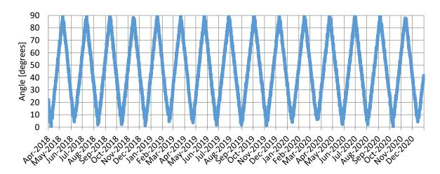
Figure 14. Evolution of the angle between MEX and TGO orbit planes from April 2018 to December 2020, as measured at the Mars equatorial plane during spacecraft equator crossings. The minimum angles correspond to the MEX-TGO orbit "quasi-alignment" periods.
