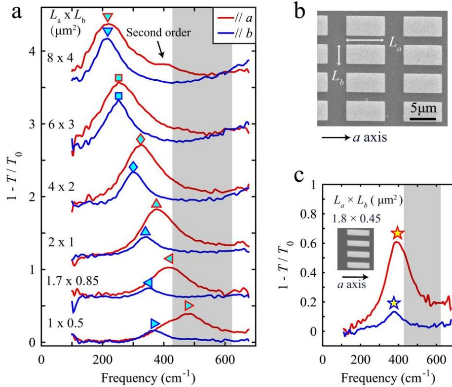
**Figure 3: Plasmon modes in the rectangle arrays on polycrystalline diamond substrates.**
