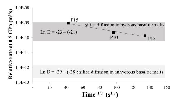
**Figure 4.** 'Relative' rates (in  $m^2/s$ ) of the serpentinite assimilation by the basaltic melt at 1300°C and 0.5 GPa versus the run duration (in  $s^{1/2}$ ). Table 5 demonstrates the applied calculation method for the "relative dissolution rate".
