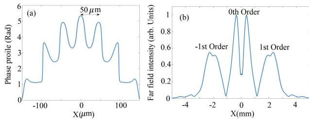
FIG. 6: (Color online)(a)Phase profile of the beam at the end of the geometric phase grating. (b) Far field intensity after the crystal end.
