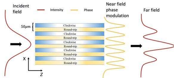
FIG. 5: (Color online) Schematic drawing of the grating simulation. Each segment of poling in the  $x$  direction corresponds to clockwise rotation and round-trip motion in parameter space. The period of each segment is set to be  $\Lambda = 50 \mu\text{m}$ .
