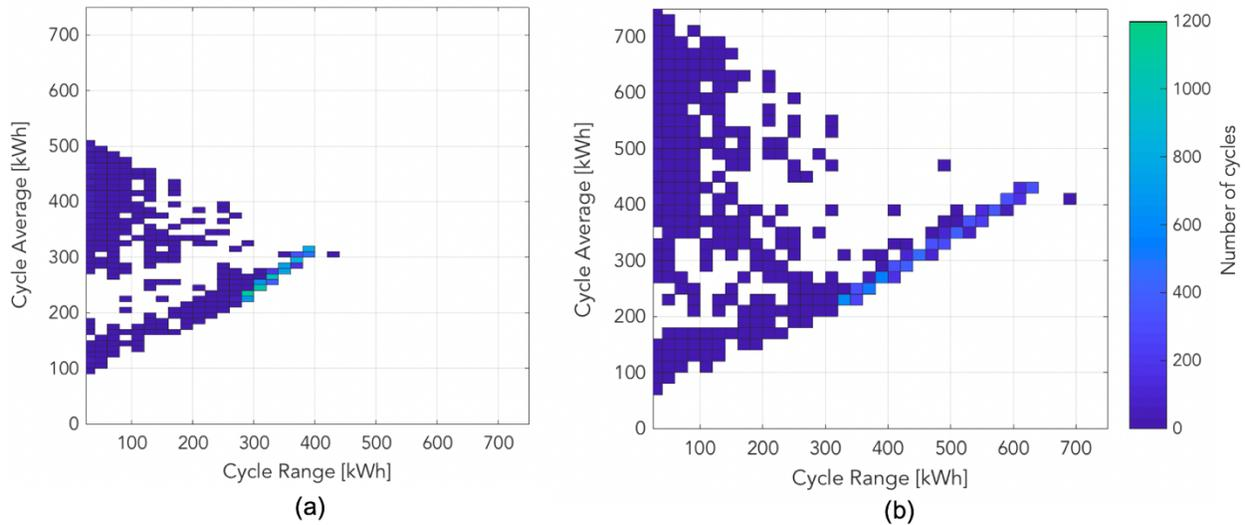
Figure 5: The number of cycles binned by cycle range and cycle average modeled over 20 years of a project life for (a) a 65–15% and (b) a 95–15% SOC limit control policies, respectively.
