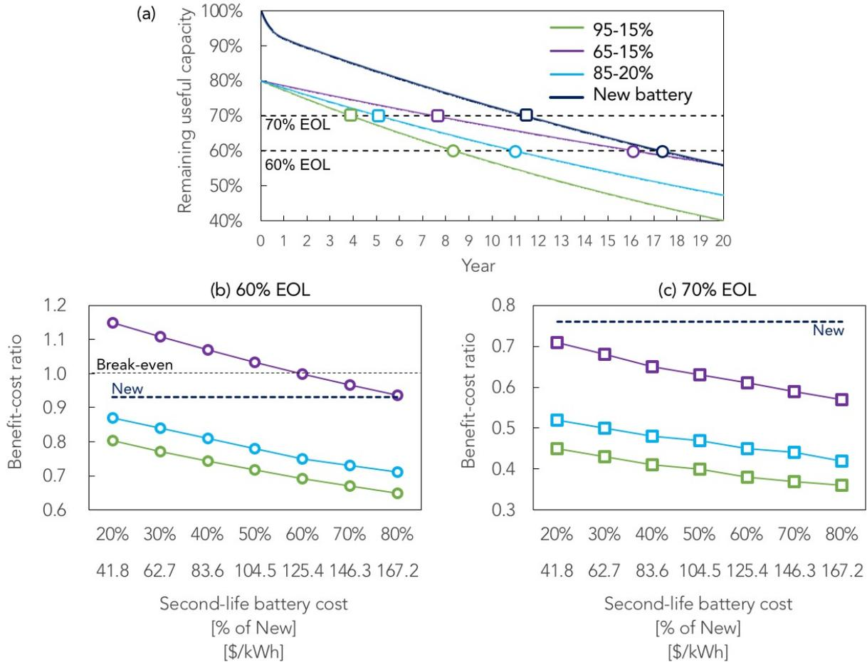
Figure 4: (a) The remaining useful capacity of the modeled batteries considering different control policies for the second-life batteries where open squares mark the 70% EOL and open circles mark the 60% EOL, (b) the benefit-cost ratio for each control policy modeled versus the capital cost to install the second-life batteries for the 60% EOL assumption, and (c) for the 70% EOL assumption.
