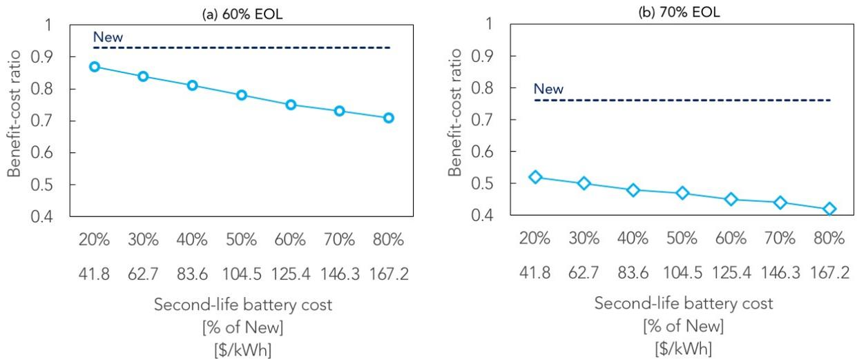
Figure 3: The benefit-cost ratio of the modeled second-life energy storage projects versus the capital cost to install the second-life batteries for the (a) 60% and (b) 70% EOL cases.
