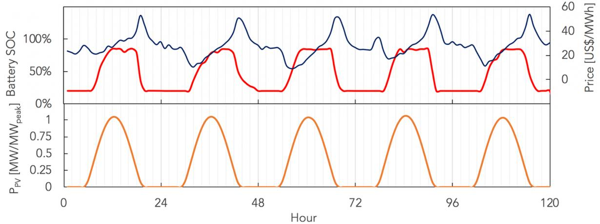
Figure 1: Sample of the power produced by the photovoltaic power plant (orange), the day-ahead spot market price (navy) and resulting optimized charge/discharge profile (red) of the energy storage system for 5 days.
