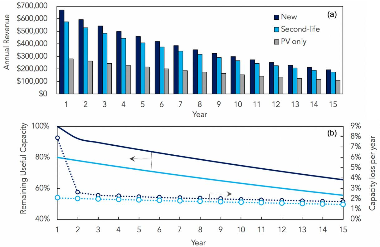
Figure 2: (a) The annual revenue of a stand-alone merchant photovoltaic power plant (PV only) and a photovoltaic + energy storage systems using new or second-life batteries, and (b) the remaining useful capacity of the batteries versus time and annual capacity fade for both energy storage projects modeled.
