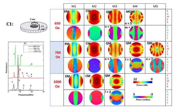
Fig. 6: Power (top row) and phase (bottom row) profiles of the resonant spin wave modes on the surface of the nanomagnet with defect of type C1 at three different bias magnetic fields. No new mode is spawned and none is quenched by the defect.
