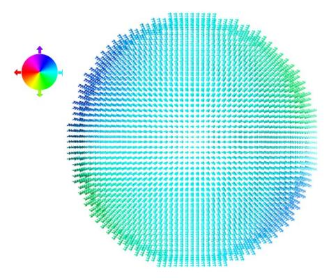
Fig. S12: Steady state micromagnetic distributions in all layers of the defective nanomagnet C4. The magnetic field is 650 Oe and is directed to right along the horizontal axis.
