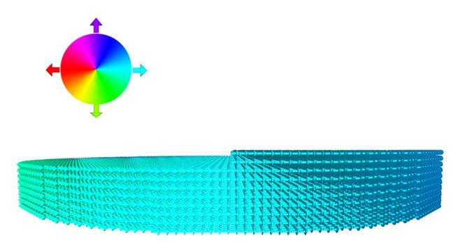
Fig. S7: Side view of the steady state micromagnetic distributions in all layers of the defective nanomagnet C2. The magnetic field is 650 Oe and is directed to right along the horizontal axis.
