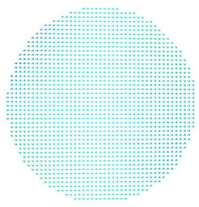
Fig. S1: Steady state micromagnetic distributions in the top layer of the defect-free nanomagnet (C0). The magnetic field is 650 Oe and is directed to right along the horizontal axis.
