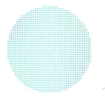
Fig. S16: Steady state micromagnetic distributions in the top layer of the defective nanomagnet C6. The magnetic field is 650 Oe and is directed to right along the horizontal axis.
