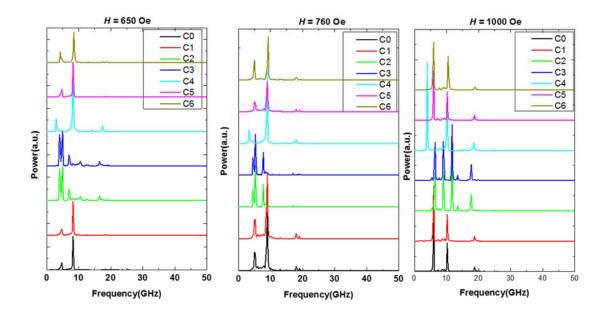
Fig. 4: Fast Fourier transforms of the  $\overline{M}_{z}(t)$  versus t oscillations for the seven different nanomagnets at three different bias field strengths (H). These are the frequencies of the dominant spin wave modes in the nanomagnets at the corresponding bias field.
