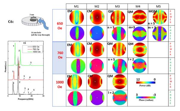
Fig. 11: Power (top row) and phase (bottom row) profiles of the resonant spin wave modes on the surface of the nanomagnet C6 at three different magnetic fields. A new mode is spawned at the low field and one is quenched at the intermediate field.
