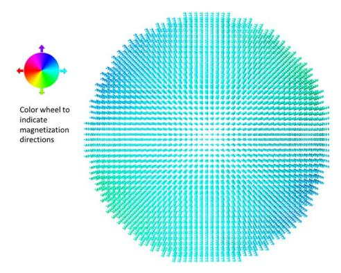
Fig. S2: Steady state micromagnetic distributions in all layers of the defect-free nanomagnet (C0). The magnetic field is 650 Oe and is directed to right along the horizontal axis.
