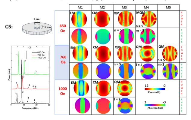
Fig. 10: Power (top row) and phase (bottom row) profiles of the resonant spin wave modes on the surface of the nanomagnet C5 at three different magnetic fields. No new mode is spawned and none quenched.
