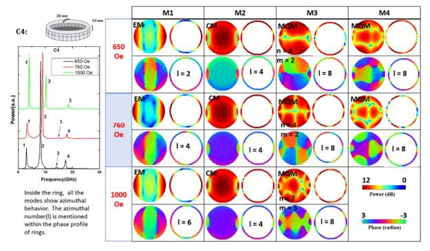
Fig. 9: Power (top row) and phase (bottom row) profiles of the resonant spin wave modes on the surface of the nanomagnet with defect C4 at three different bias magnetic fields. This is the case that most closely approximates the structure in Fig. 1. Here, we show, separately, the power and phase profiles in the surface of the nanomagnet (left) and in the surface of the 20 nm thick annulus (right). No new mode is spawned, but one is quenched.
