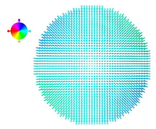
Fig. S14: Steady state micromagnetic distributions in all layers of the defective nanomagnet C5. The magnetic field is 650 Oe and is directed to right along the horizontal axis.
