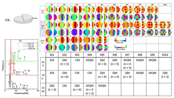
Fig. 8: Power (top row) and phase (bottom row) profiles of the resonant spin wave modes on the surface of the nanomagnet with defect C3 at three different bias fields. The left panel shows the Fourier transform spectra  $\tilde{M}^{z_m}(f, x, y)$  at three different bias magnetic fields. New resonant modes are spawned by this defect.
