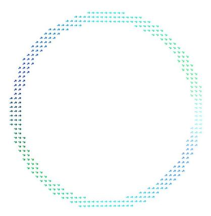
Fig. S11: Steady state micromagnetic distributions in the top layer of the defective nanomagnet C4. The magnetic field is 650 Oe and is directed to right along the horizontal axis.
