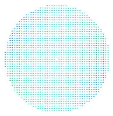
Fig. S3: Steady state micromagnetic distributions in the top layer of the defective nanomagnet C1. The magnetic field is 650 Oe and is directed to right along the horizontal axis.
