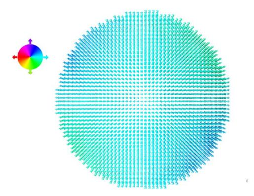
Fig. S6: Steady state micromagnetic distributions in all layers of the defective nanomagnet C2. The magnetic field is 650 Oe and is directed to right along the horizontal axis.
