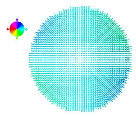
Fig. S9: Steady state micromagnetic distributions in all layers of the defective nanomagnet C3. The magnetic field is 650 Oe and is directed to right along the horizontal axis.
