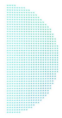
Fig. S5: Steady state micromagnetic distributions in the top layer of the defective nanomagnet C2. The magnetic field is 650 Oe and is directed to right along the horizontal axis.
