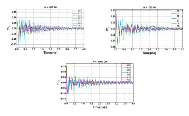
Fig. 3: The spatially averaged out-of-plane magnetization component as a function of time for the seven different (defect-free and defective) cobalt nanomagnets. The plots are for three different bias fields of strength 650 Oe, 760 Oe and 1000 Oe.
