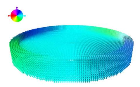
Fig. S13: Side view of the steady state micromagnetic distributions in all layers of the defective nanomagnet C4. The magnetic field is 650 Oe and is directed to right along the horizontal axis.
