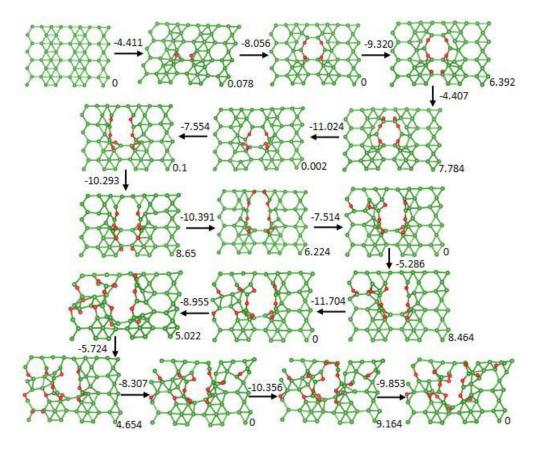
**Figure 2.** Optimized atomic structure of the first steps of the oxidation process of boron sheet of  $\chi$ -type. The numbers near the arrows is formation energies (in eV) and numbers in the corner of the structures is total magnetic moment of the supercell (in  $\mu_B$ ).
