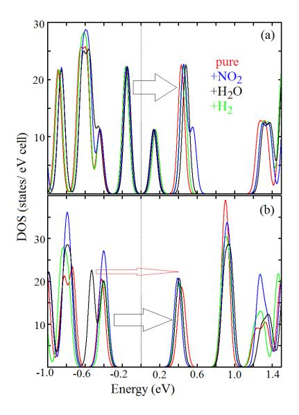
**Figure 5.** Total densities of states of  $\beta$ -OBS (a) and  $\chi$ -OBS (b) before (red) and after adsorption of nitrogen dioxide (blue), water (black) and hydrogen (green) molecules. Arrows are indicating possible optical transitions influenced by adsorption of the molecules.
