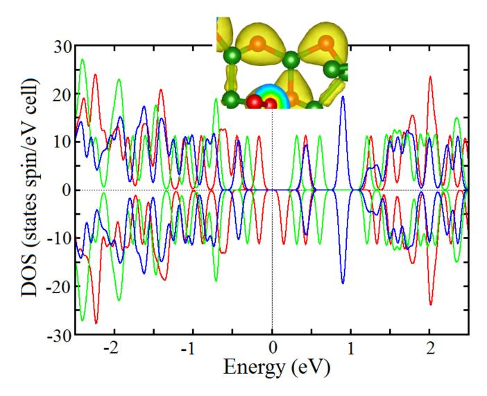
**Figure 4.** Spin-polarized density of states of fully oxidized boron sheet of  $\beta$ -type (red line) and  $\chi$ -type (blue line). Green line is corresponding with  $\beta$ -OBS after passivation of magnetic center by hydrogen (Fig. 3a). Charge density distribution in the part of oxidized  $\beta$ -OBS are shown on inset.
