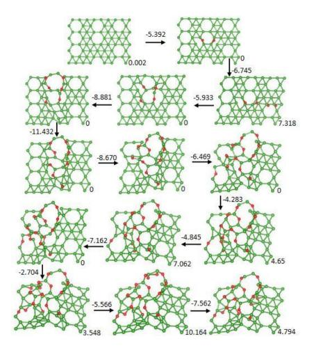
**Figure 1.** Optimized atomic structure of the first steps of the oxidation process of boron sheet of  $\beta$ -type. The numbers near the arrows is formation energies (in eV) and numbers in the corner of the structures is total magnetic moment of the supercell (in  $\mu_B$ ).
