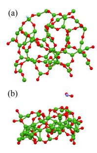
**Figure 3.** Optimized atomic structure of totally oxidized boron sheet of  $\beta$ -type with magnetic center passivated by hydrogen atom (a) and totally oxidized boron sheet of  $\chi$ -type with physically adsorbed molecules of NO<sub>2</sub>.
