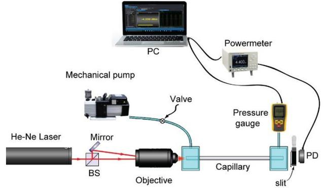
Fig 2. Schematic of the experimental setup of the gas refractometer. BS: beam splitter; PD: photodiode.
