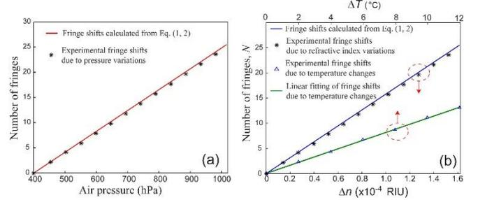
Fig 4. (a) Fringe shifts in response to variations in air pressure in the capillary core, (b) Fringe shifts in response to variations in the refractive index of gas filled in the capillary as well as variations in surrounding temperatures.
