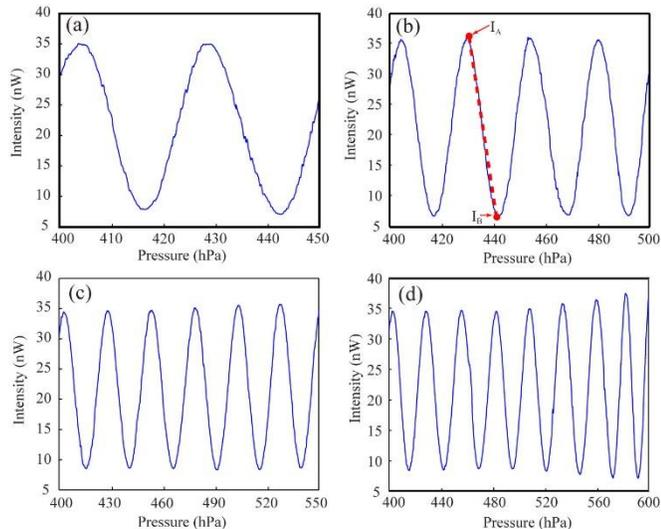
Fig. 5 Intensity variations measured by a photodiode detector behind a slit, when the air pressure in the capillary core changes from 400 hPa to (a) 450 hPa, (b) 500 hPa, (c) 550 hPa, and (d) 600hPa.
