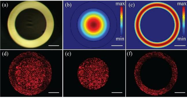
Fig. 1. (a) microscopic image of the cross section of the capillary, (b) fundamental mode guided by the capillary core, (c) fundamental mode guided by the capillary cladding, output intensity of the capillary when laser is coupled to (d) both of the core and cladding, (e) only the hollow core and (f) only the cladding. The scale bar in each image has a length of 100  $\mu\text{m}$ .
