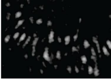
Fig 3. Interferogram partially captured by a CMOS camera at the output end of the capillary, while the inner air pressure of the capillary elevates from 400 to 1012 hPa.
