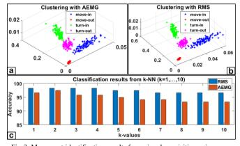
Fig.3: Movement identification results from signal acquisition using: a-b) k-means (k=4) clustering with AEMG and RMS; c) k-NN classification
