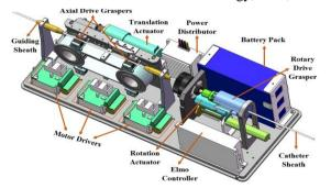
Fig. 1: CAD model of robotic system for cardiovascular intervention.
