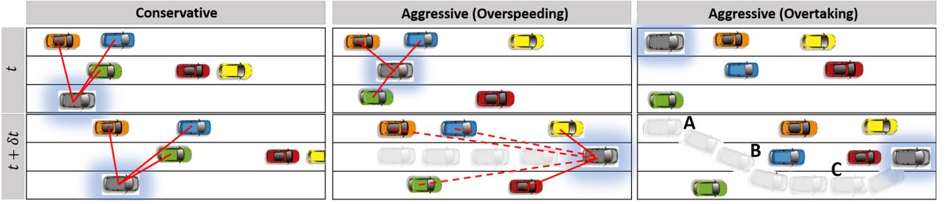
(a) In all three scenarios, the ego-vehicle is a gray vehicle marked with blue glow. (left) A conservative vehicle, (middle) overspeeding vehicle in the same lane, and (right) weaving and overtaking vehicle.
