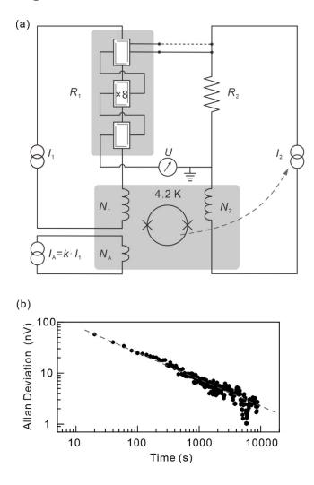
Fig. 2 (a) Schematic diagram of the cryogenic current comparator resistance bridge for precision measurements of  $R_{xy}$  (configured by solid line) and  $R_{xx}^{\text{single}}$  (configured by dotted line). Read details in main text. (b) Allan deviation of the bridge voltage difference, acquired for 10 hours at the magnetic field of 10 T and temperature of 2 K. It follows the inverse square root time dependence  $(1/\sqrt{\tau})$  of white noise up to the sampling time of  $10^4$  s.
