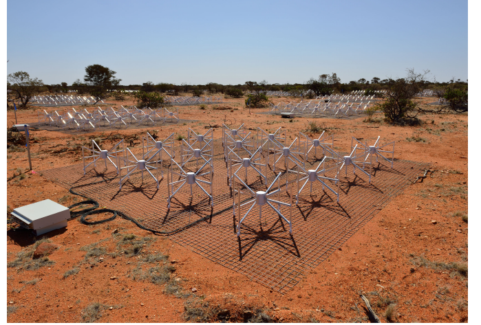
Figure 1. An MWA tile connected to a beamformer (white rectangular box). Each antenna element contains an LNA in the central hub (white cylindrical container). Photo credits: Curtin University and MWA Collaboration.
