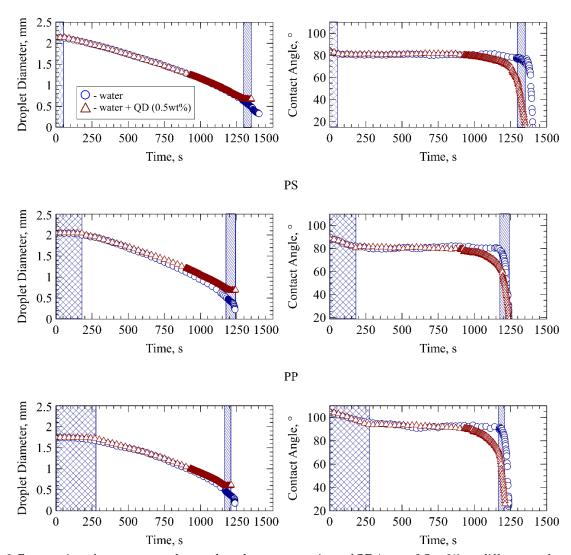
**Figure 2.** Evaporation of pure water and water-based nanosuspensions of QD ( $c_{QD} = 0.5$  wt%) on different surfaces: HDMS ( $\theta_w = 84^\circ$ ), PS ( $\theta_w = 90^\circ$ ) and PP ( $\theta_w = 106^\circ$ ). Crossed areas on each graph correspond to CCR evaporation mode and slant-lined areas correspond to ACCR (Additional Constant Contact Radius) mode caused by the coffee stain formation on the droplet periphery. Volume of droplet deposited is 2.2  $\mu l$ .
