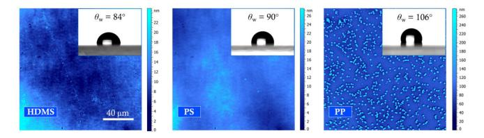
**Figure 1.** Topography of surfaces (squares 160  $\mu m \times 160 \mu m$ ) investigated with Confocal Profilometer  $\mu$ Surf (NanoFocus Expert), inner microphotographs illustrate static wetting by water droplet (2.2  $\mu l$ ). From left to right: HDMS ( $\theta_w = 84^\circ$ ), PS ( $\theta_w = 90^\circ$ ) and PP ( $\theta_w = 106^\circ$ ).
