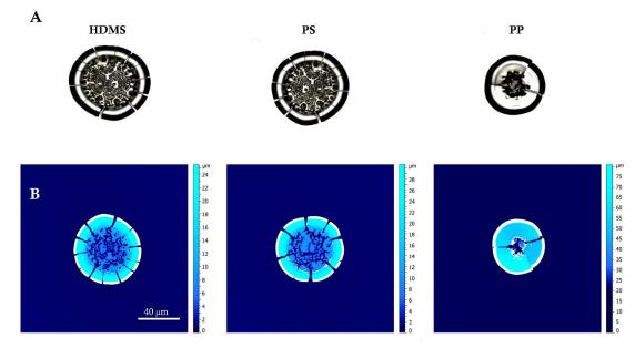
**Figure 4.** Deposits formed evaporation of water-based nanosuspensions of QD (0.5 wt%) on surfaces with different wettability: HDMS ( $\theta_w = 84^\circ$ ), PS ( $\theta_w = 90^\circ$ ) and PP ( $\theta_w = 106^\circ$ ). A: confocal microphotographs show the deposition patterns left after complete drying of nanofluids. B: the topography maps of the coffee stains. The size of each square 1.6 *mm* × 1.6 *mm*. Volume of droplet deposited is 2.2 µ*l*.
