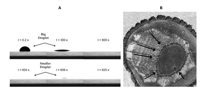
**Figure 9.** A: Time-lapse images of spreading and evaporation of Silwet L-77 CAC aqueous solution with QDs ( $c_{QD} = 0.5 \text{ wt\%}, c_{ss} = CAC < CWC$ ) on HDMS surface. The image sequence shows formation of inner coffee ring. Volume of droplet deposited is 2.1  $\mu$ l. B: Topography reconstructed from height-position matrix obtained by confocal profilometer (PS substrate). Receding TCL traces are shown by black arrows.
