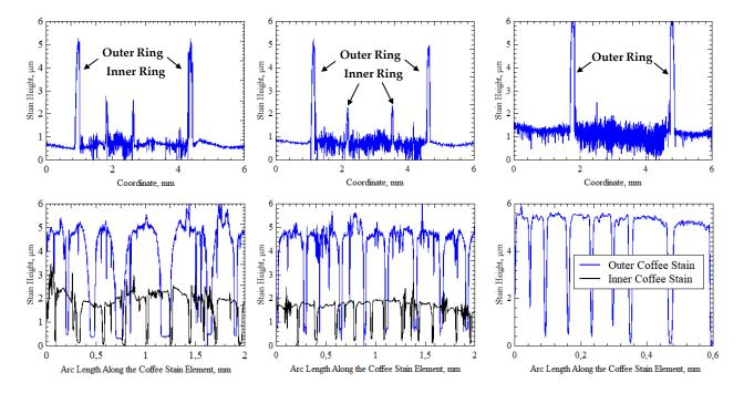
**Figure 10.** Morphology and crack structure of deposition patterns left after drying of trisiloxan-laden nanosuspensions of QDs (0.5 wt%) on surfaces with different hydrophobicity: HDMS ( $\theta_w = 84^\circ$ ), PS ( $\theta_w = 90^\circ$ ) and PP ( $\theta_w = 106^\circ$ ) obtained with use of confocal profilometry. A: Coffee stain profiles. B: Cracks distribution along the coffee stains.
