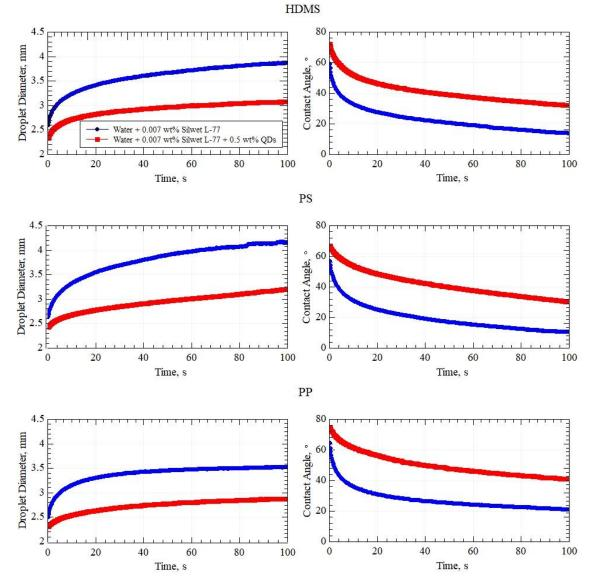
**Figure 6.** Wetting behavior of Silwet L-77 CAC aqueous solutions with ( $c_{QD} = 0.5$  wt%,  $c_s = CAC < CWC$ , denoted by red markers) and without ( $c_s = CAC < CWC$ , denoted by blue markers) QDs on different hydrophobic surfaces: HDMS ( $\theta_w = 84^\circ$ ), PS ( $\theta_w = 90^\circ$ ) and PP ( $\theta_w = 106^\circ$ ). Volume of droplet deposited is 2.2  $\mu l$ .
