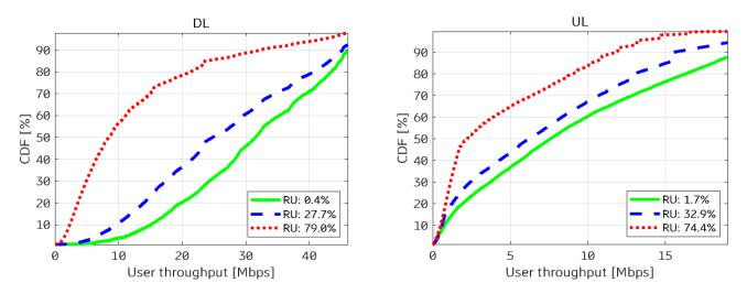
Figure 3: Throughput distributions under different traffic loads in an NR A2G system at the low band.
