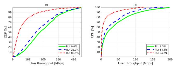
Figure 4: Throughput distributions under different traffic loads in an NR A2G system at the mid-band.
