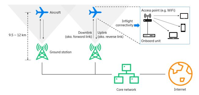
Figure 1: An illustration of the system architecture for cellular-based direct A2G communications.
