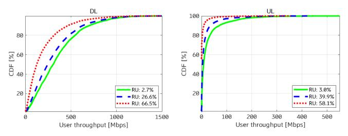
Figure 5: Throughput distributions under different traffic loads in an NR A2G system at the high band.
