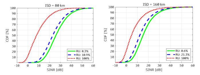
Figure 2: Downlink SINR distributions under different traffic loads in an NR A2G system at the low band.
