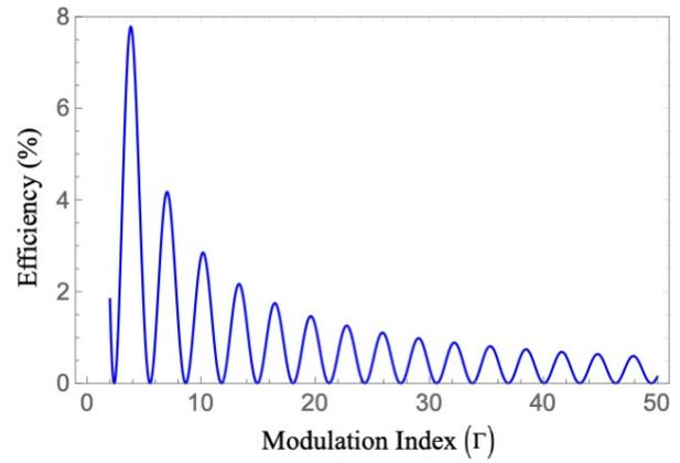
**Fig. 5.** Power conversion efficiency at port C as obtained from Eqs. (12). With  $\delta\omega T = \delta/\Gamma$ , the efficiency is independent of  $\delta$ . Other parameters are the same as in Fig. 1.
