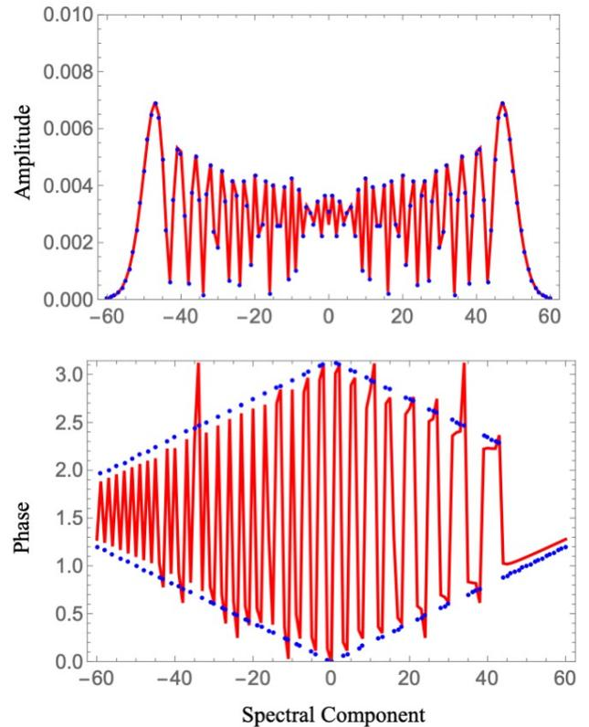
**Fig. 3.** Amplitude and absolute value of the phase of spectral components at port C. The red curve is the result of the solution of 241 linear equations, Eqs. (1-2). The blue dots are the approximate solution, Eq. (11). Parameters are identical to Fig. 1.
