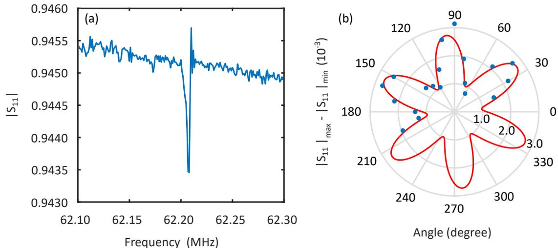
FIG. A1. IDT alignment. (a)  $S_{11}$  signal obtained during the IDT alignment. The external coupling of the acoustic WGM can be obtained from the magnitude of the dip in the signal. (b)  $S_{11}$  dip magnitude as a function of the crystal rotation along the  $c$ -axis. The IDT is placed at one of the 6-fold external coupling maxima.
