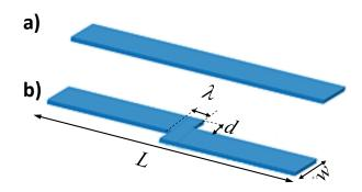
**Figure 1.** (a) Conventional nanowire with length L and width *w* and (b) Nanowire with a stepped area at its center with dimensions *d* and  $\lambda$  to pin the DW.
