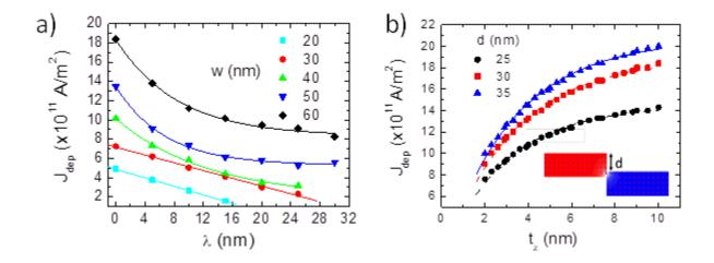
Figure 3. (a) Plots of  $J_{dep}$  versus the step width  $\lambda$  for various widths of nanowire w. For the plots, d was fixed to w/2. (b)  $J_{dep}$  versus the nanowire thickness  $t_z$  for d = 25, 30 and 35 nm and  $\lambda = 0$ .
