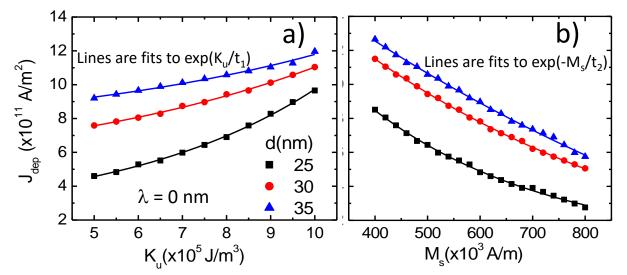
Figure 4. Domain wall depinning current density versus (a)  $K_u$  and (b)  $M_s$  for different values of d. The lines are fit to exponential growth function for case (a) and exponential decay for case (b). The nanowire length and width are fixed to 200 nm and 40 nm, respectively.
