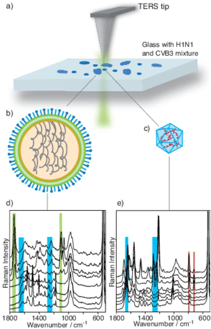
Figure 1: a) Schematics of the transmission TERS setup used in the experiments with the virus mixture spread on a slide and the laser illuminating the sample from below. b) Model of H1N1 virus with protein spikes (blue) protruding from the lipid bilayer (green). c) Model of a CVB3 virus with the protein lattice (blue) on the surface and RNA strands (red) inside the virus. d) Selected TERS spectra recorded on H1N1 virus. e) Selected TERS spectra recorded on CVB2 virus. In d) and
