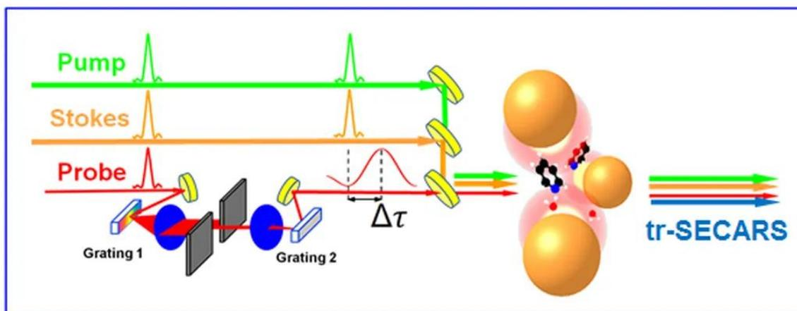
Figure 2: Simplified experimental setup of time-resolved surface-enhanced CARS spectroscopy.
